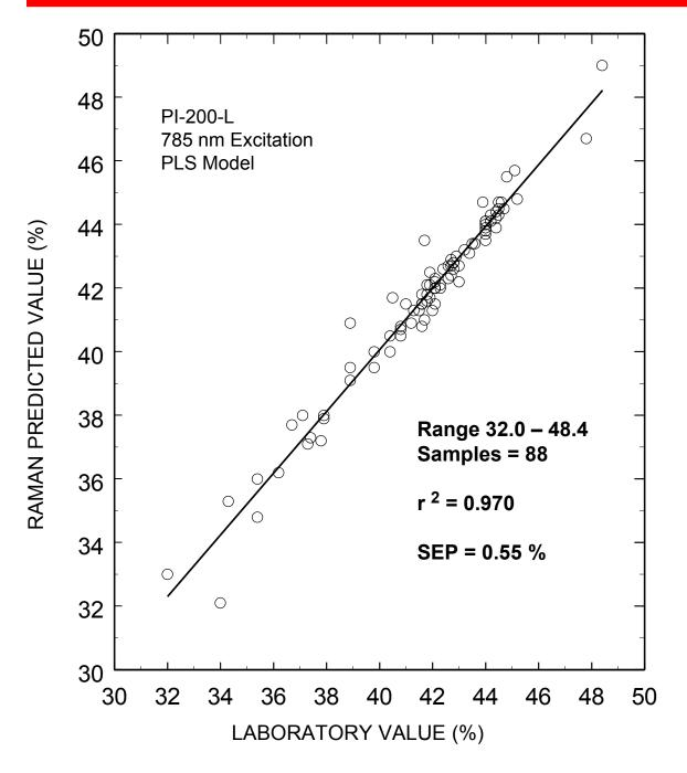
Typical on-line partial least squares (PLS) analysis of the MDEA concentrations. The plot shows Raman predicted values vs. the measured laboratory values. The standard error of prediction for the PLS model with outliers removed was 0.55 %.
