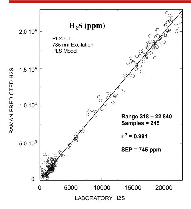
Typical on-line partial least squares (PLS) analysis of the H2S (ppm) concentrations. The plot shows Raman predicted values vs. the measured laboratory values. The standard error of prediction for the PLS model with outliers removed was 745.
