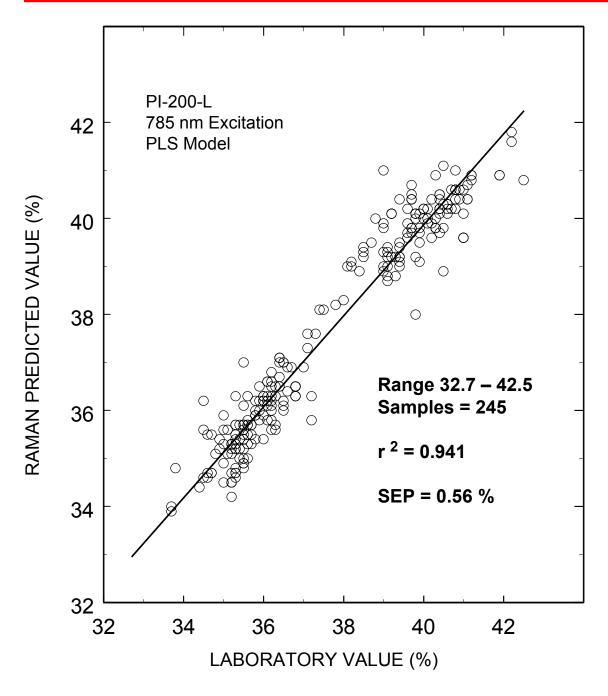
Typical on-line partial least squares (PLS) analysis of the DGA concentrations. The plot shows Raman predicted values vs. the measured laboratory values. The standard error of prediction for the PLS model with outliers removed was 0.56 %.
